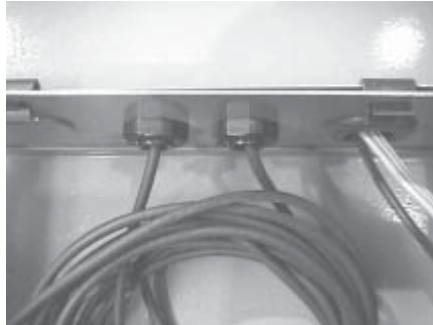
Inside of electronics box: threaded rings for sensor cable
