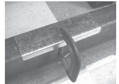
Drill guide in place
